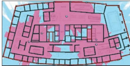
Figure 2. Sensor Coverage View—Determine security sensor coverage for your risk profile
